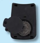
Carefully remove screw from battery cover and remove batteries. Install new batteries using the correct polarity. Use only CR-2325 or equivalent.
